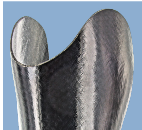
Composite on outside of lay-up
