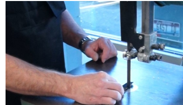
7. Cut the strut on your mark. Cut it with a bandsaw, scissors or a hot knife.
