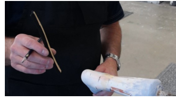
3. Figure out the curve of the strut and how it best fits on the cast.
