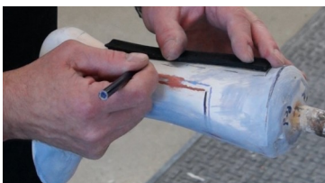
9. Mark your distal and your proximal. Put some dashes in for the width.
