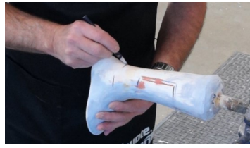
2. Split the difference between the two ankle centers and put the base of the strut at midline with the medial and at the peak of the proximal on the lateral.
