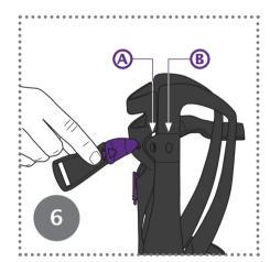
Push the buckle out of the lower shell and into the desired position.
